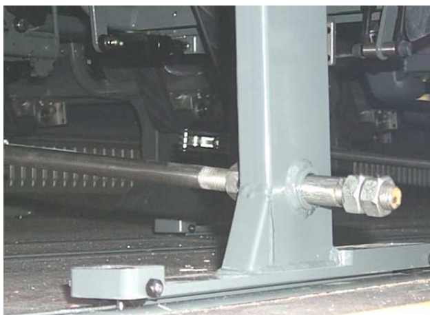
Figure 12: Push/pull rod in the fully locked position. Operating lever fully forwards
