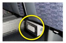
Dual outlets are mounted under the front of the seat between the passengers to ensure neither passenger is inconvenienced by the outlet location. Stainless steel mounting bracket and faceplate with
