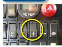
Dash mounted control switch that matches the OE switches on 2007 and newer Van Hool C and T models only.
