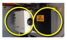
Circuit breaker panel w/GFCI protection and power indicator lights. Distributes power to 4-6 circuits instead of only 1 as is typical for inverter outputs on 2007 or newer Van Hool C and T models.
