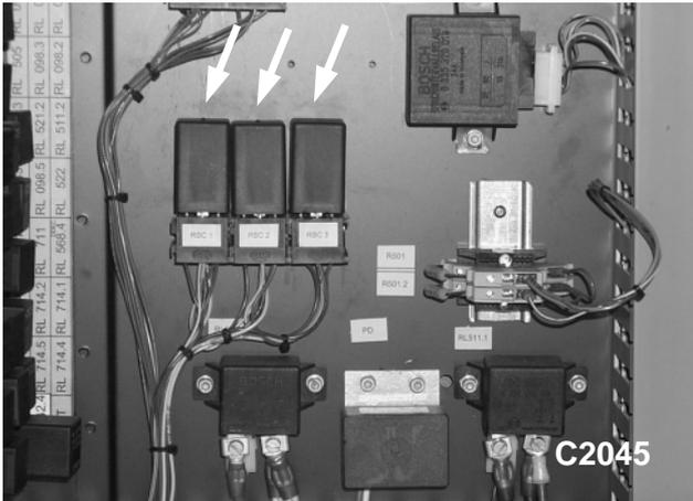
**Figure 1: C2045 brake pad wear indicator relays (from left to right):**
