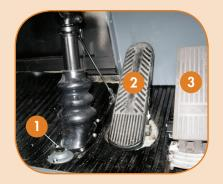
DRIVER'S FLOORBOARD AREA Steering column control 2 Brake 3 Accelerator
