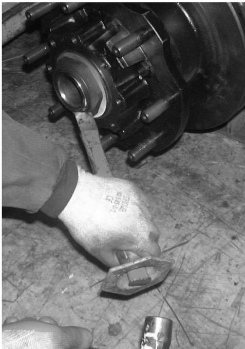
**Figure 5: Staked nut bending procedure**
