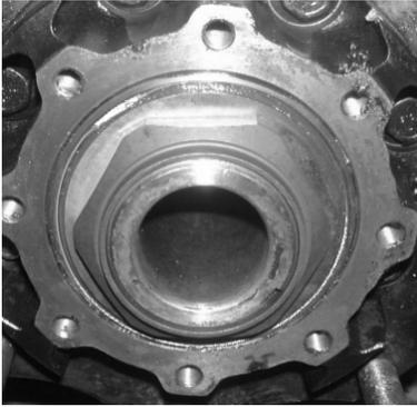
**Figure 4: Hub nut and tang washer fully up**
