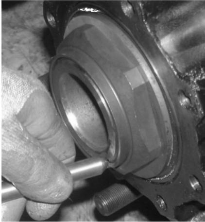
**Figure 6: Bending out of the staked part of the hub nut**
