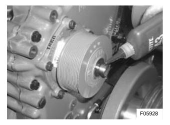
Figure 8: Applying thread locking adhesive
