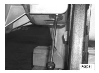
9) Tighten the pulley nut to a torque of 295 ft.lbf (400 Nm) as shown in Figure 12.
