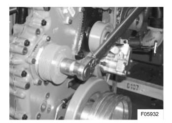
Figure 12: Torqueing pulley retaining nut
