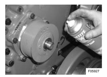
Figure 7: Degreasing the thread
