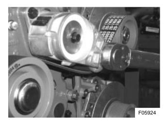
Figure 3: Lifting the belt tensioner
