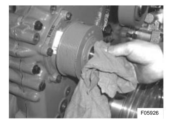
Figure 6: Removing debris with a clean cloth
