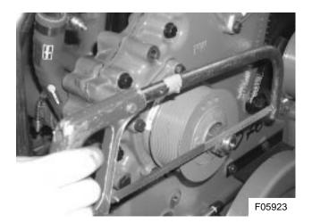
Figure 4: Cutting the shaft
