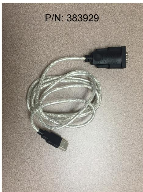
Knorr-Bremse UDIF diagnostic interface. This device allows communication between the coach and a laptop running the NEO software.
