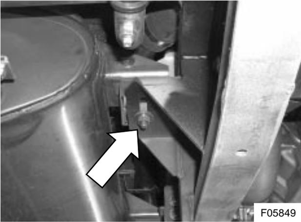
**Figure 8: Right-hand rear most muffler rubber isolator mount nut**
