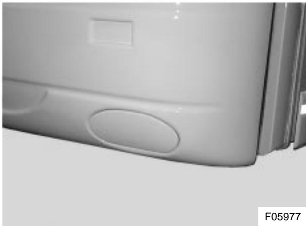
**Figure 2: Lamp recess plug flush with bumper skin (C2045)**
