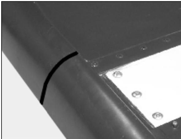
**Figure 4: Gap sealed w/ Sikaflex® 222**
