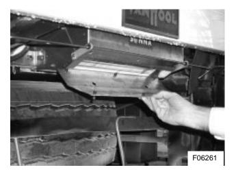
Figure 3: HVAC front air filter access door
