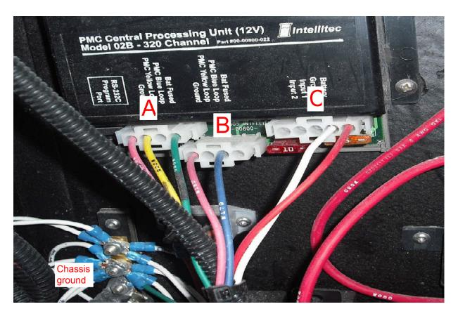
System communication voltage should be between 7 and 9 volts (DC). Voltage is generated by the CPU Module. Voltage is checked with connectors plugged in.
