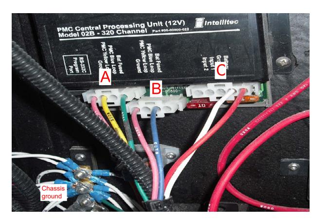
System communication voltage should be between 7 and 9 volts (DC). Voltage is generated by the CPU Module. Voltage is checked with connectors plugged in.
