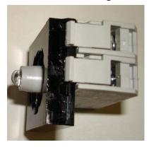
Install switch assembly to the push button that's installed in dash.
