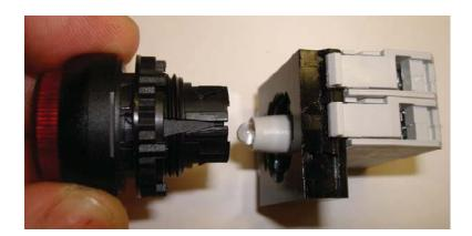
Once switch mount is in place turn the lock then ready for wires to be hooked up. Refer to wire diagram if needed.
