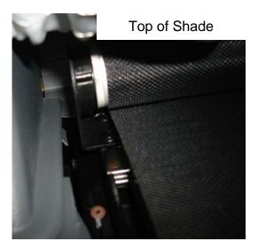
Use flat tip screw driver to unlock shade for removal.
