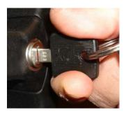
Step 5: Apply a little side pressure and pull the cylinder out.
