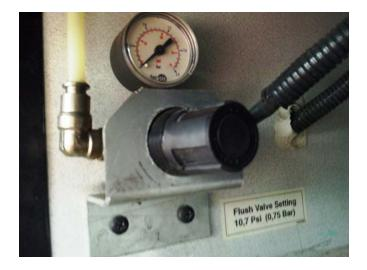
With full air pressure on coach, turn clockwise to increase pressure or counterclockwise to decrease pressure. The pressure setting should be between 11 to 14 psi max. After setting the pressure push knob back to the lock position. Flush the toilet to verify proper operation, re-adjust air pressure if necessary for better operation.
