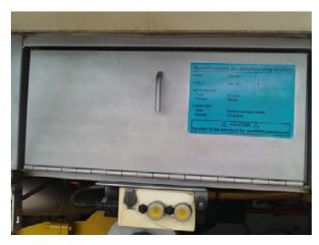
The lavatory air pressure regulator is located in the engine compartment behind the service door.
