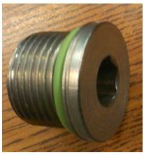
12 MM Allen to remove from engine block.
