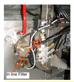
The rear inline filter is located on the front wall of the drive axle cavity above the drive axle service brake relay valve
