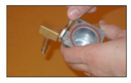
Screw the restrictor nipple on the solenoid valve as shown in figure.
