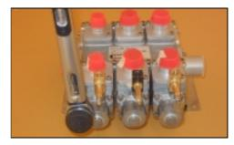
**25.** Tighten the Banjo screws to a torque of 5 ft.lbf (7Nm), using a torque wrench with a 14-mm socket.
