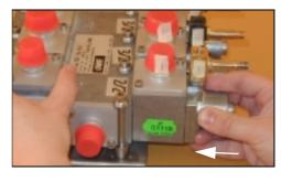
**19.** Screw the Allen screws loosely to make it easier to fit the Banjo couplings. These screws must be torqued in step 25.
