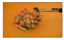
**26.** Reinstall the solenoids by screwing the plastic nuts hand tight.
