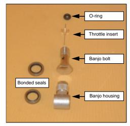
**21.** Insert the O-ring into the solenoid valve bore. Put the throttle insert into the bore with the shorter pin in the solenoid valve.
