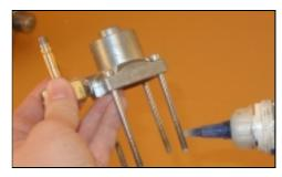
**18.** Place the valve actuator housing with the new O-ring on the valve plate, using your hand to guide it into the correct position.
