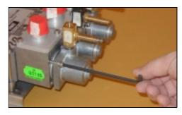
**8.** Lift off the valve actuator housing.
