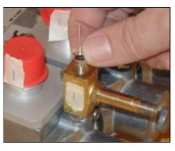
**22.** Place the Banjo bolt in the Banjo housing with the two bonded seals as shown in figure right.
