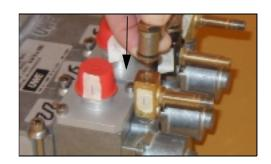
**24.** Using a torque wrench and a 4 mm hex driver, tighten the Allen bolts crosswise to a torque of 3 ft.lbf (4Nm).
