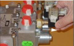
**5.** Undo and remove the air supply banjo bolts using a 14mm or 15mm box wrench.
