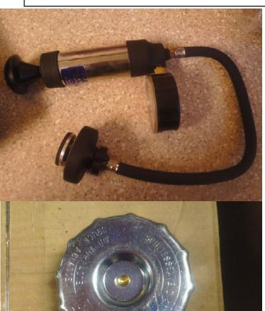
Use a cooling system pressure test tool to check the radiator and surge tank pressure caps.
