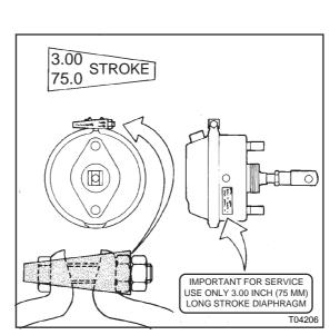
Figure 1: Labeling long stroke brake chamber of the front axle
