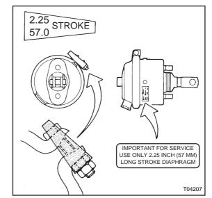
Figure 2: Labeling long stroke brake chamber of the tag axle
