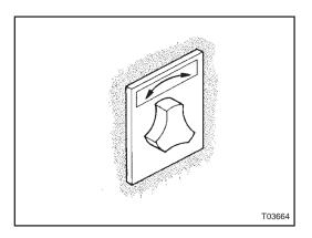
Figure 5:Rotary knob to lock entrance door from inside the coach
