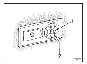
Figure 6:Outside handle of entrance door with lock (1) and rotary handle to lock/unlock (2)
