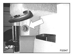
Figure 4:Location of pneumatic emergency switch, below driver's personal cabinet in stepwell
