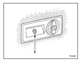
Figure 2:Outside handle of entrance door with open/close push-button switch (1)
