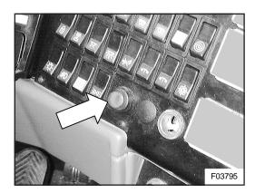
Figure 1:Location of entrance door push-button switch on right hand side control panel
