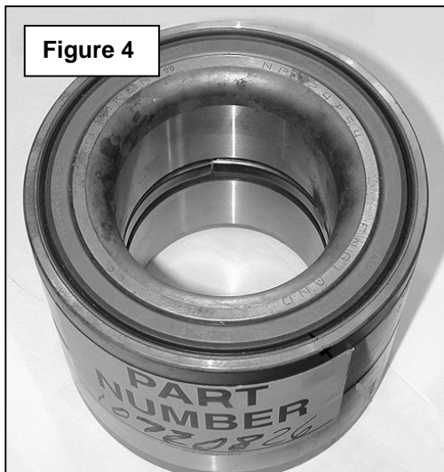
Figures 4 and 5: Both ends of the old style bearing assembly are identical.
