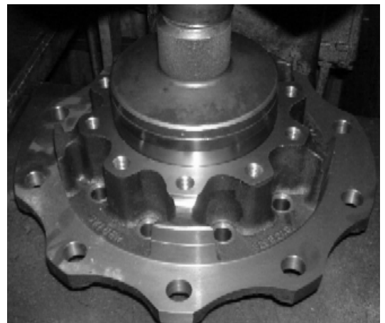
Figure 13: Bearing in hub installation – stage 2
