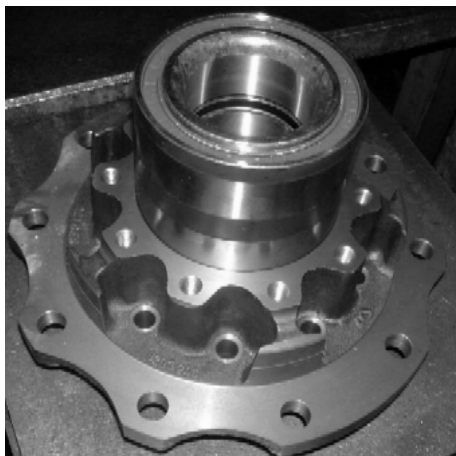
Figure 12: Bearing in hub installation – stage 1
