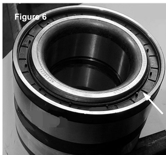
Figure 6: Outboard end of the new style wheel bearing assembly has new seal
