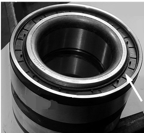
Figure 3: The outboard bearing has a new seal
