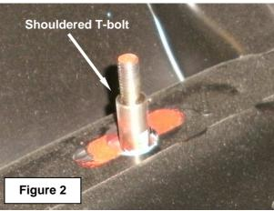
2. The bumper shell attaches to the back-up beam by means of six shouldered-type T-bolts that have been molded into the shell (Figure 2) and that pass through slots that have been machined into the beam (3, Figure 1).
