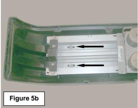
3) With the aid of an assistant, lift the bumper shell off the coach and place it upside down on a suitable work surface covered with cardboard, so as not to damage the paintwork.
