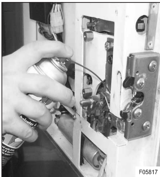
Figure 31: Door lock lubrication
