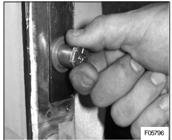
Figure 10: Trial-fitting the striker bolt base plate assembly
