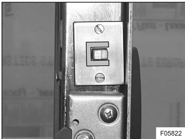
Figure 36: Dead bolt guard installation
