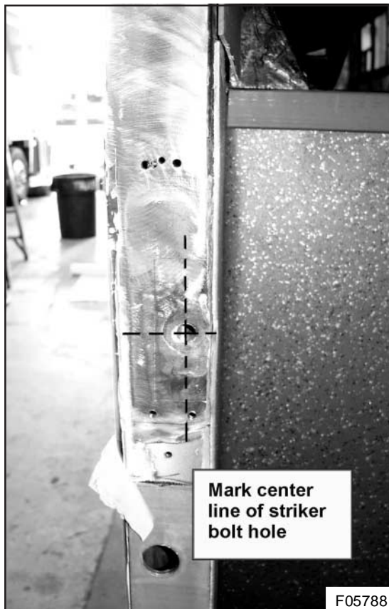
Figure 2: Striker bolt hole horizontal and vertical center lines
