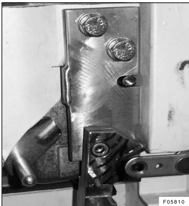
Figure 24: Door latch adapter linkage A installation (shown with hex bolts)
