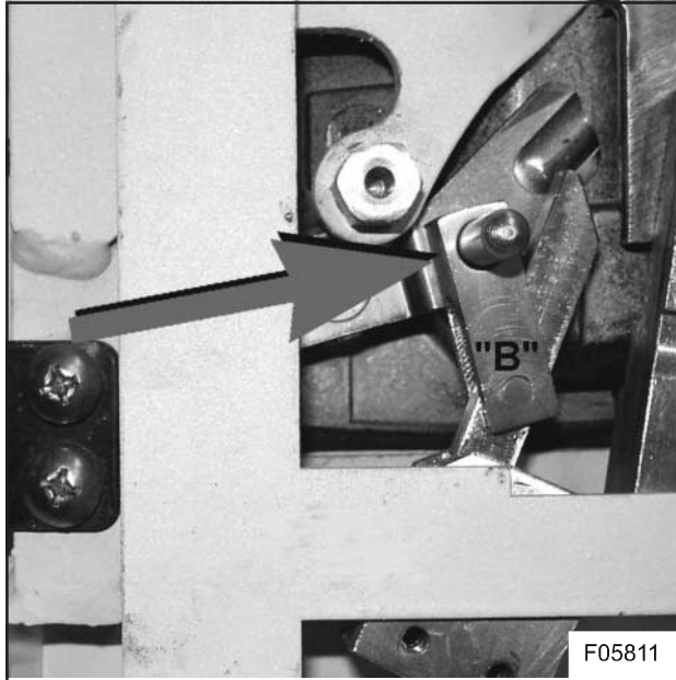
Figure 25: Adapter linkage B installation step 1
