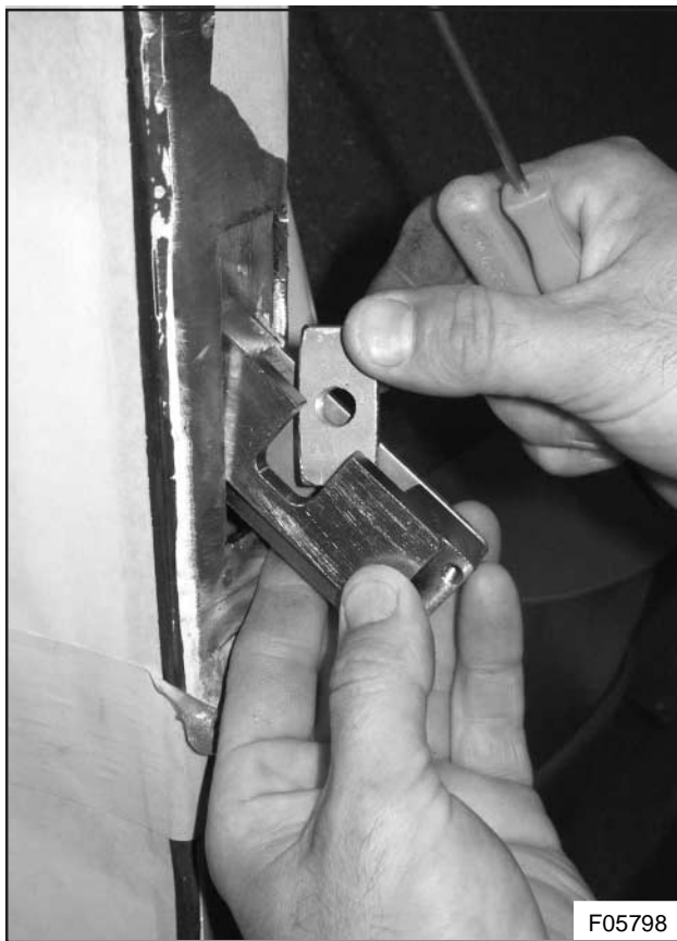
Figure 12: Base plate and striker bolt nut installation
