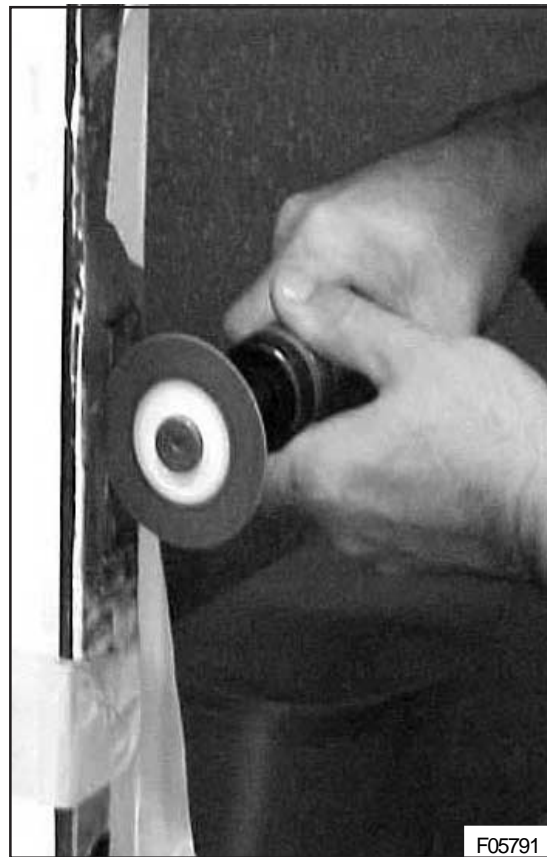
Figure 5: Cutting the B post to accept the striker bolt base plate assembly
