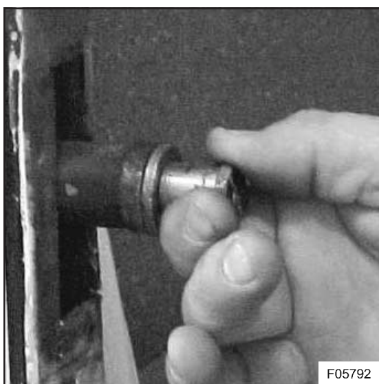
Figure 6: Striker bolt bushing removal
