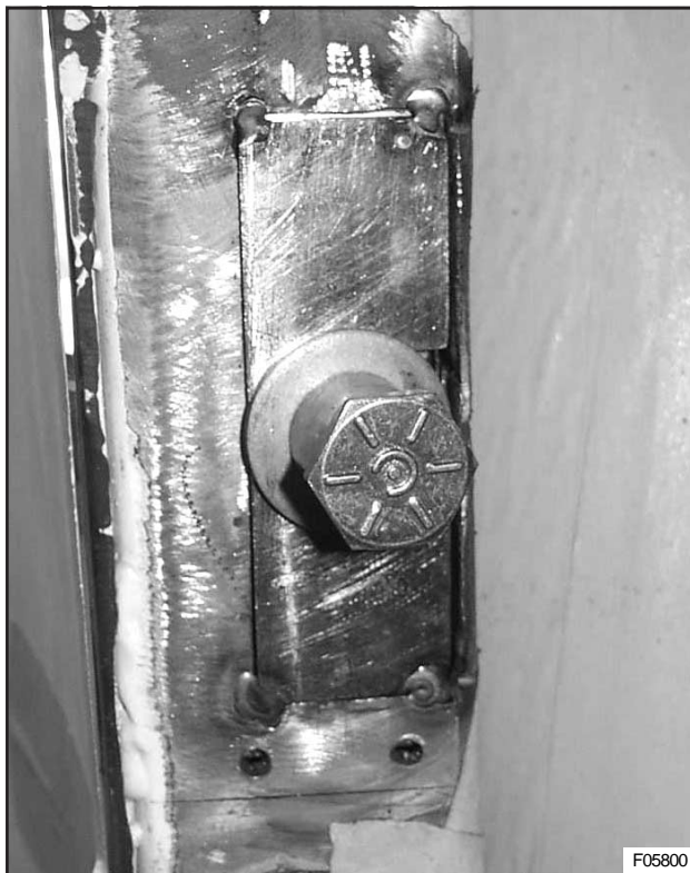
Figure 14: striker bolt base plate assembly spotwelded in place
