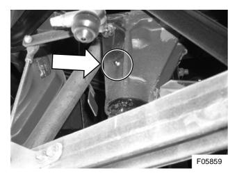
Figure 1: Steering linkage idler arm # VH R0 10538746 with grease nipple location shown
