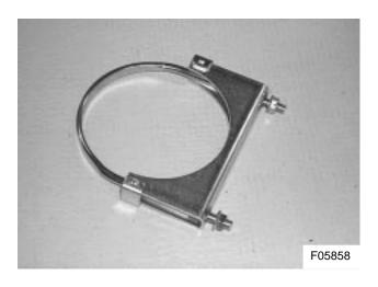
Figure 18: Clamp assembly VH 10749062
