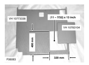
Figure 24: Modified main trim panel VH 10773338 and door lock closing panel VH 10783104
