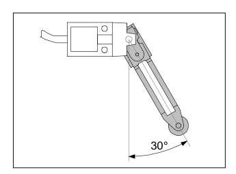
Figure 49: Roller arm position on switch shaft
