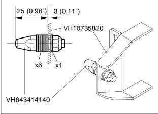
Figure 37: Guide pin brackets and mounting bolts
