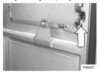
Figure 44: Rotary latch adjuster shims
