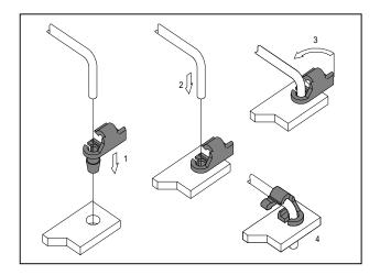
Figure 10: Snap-on rod end operation. Removal is reverse to installation
