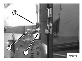
Figure 14: Lever, upper and lower connections to rotary latches.
