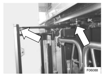
Figure 33: Tie rod ball joint location
