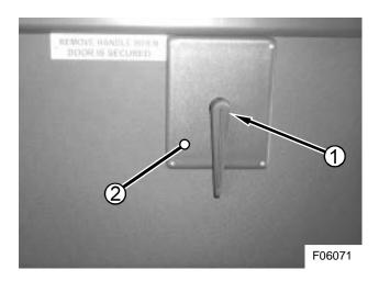
Figure 2: Emergency door handle (1) and linkage cover plate (2)
