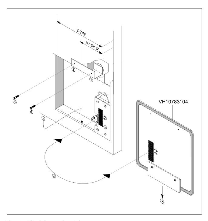
Figure 25: Trim closing panel installation
