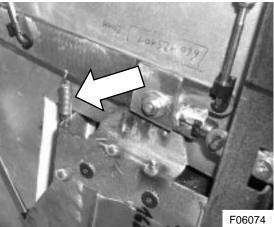
Figure 11: Emergency handle cam assembly and pull rod
