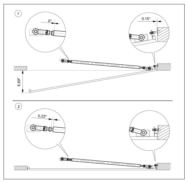
Figure 43: Parallel opening door adjustment references
