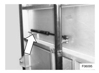
Figure 41: Gas strut installation
