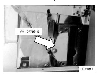
Figure 18: Door lock cam support bracket installation
