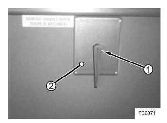
Figure 8: Emergency door handle (1) and linkage cover plate (2)
