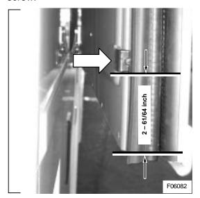
Figure 23: Proximity switch trigger installation
