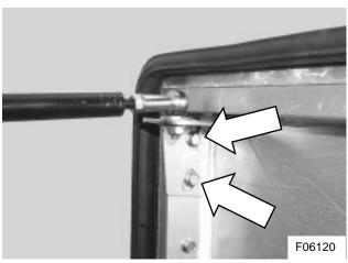
Figure 34: Tie rod mounting bracket bolts
