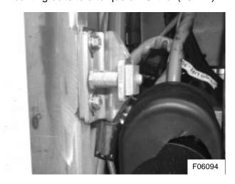
Figure 40: New striker bolt assembly installation
