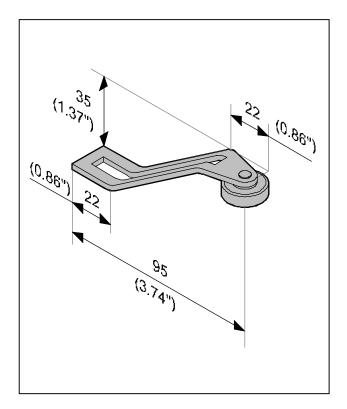
Figure 47: New shape of roller arm VH 10793025
