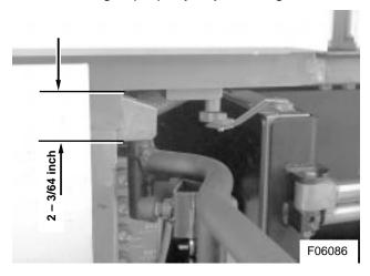
Figure 31: Upper pantograph hinge and installation distance
