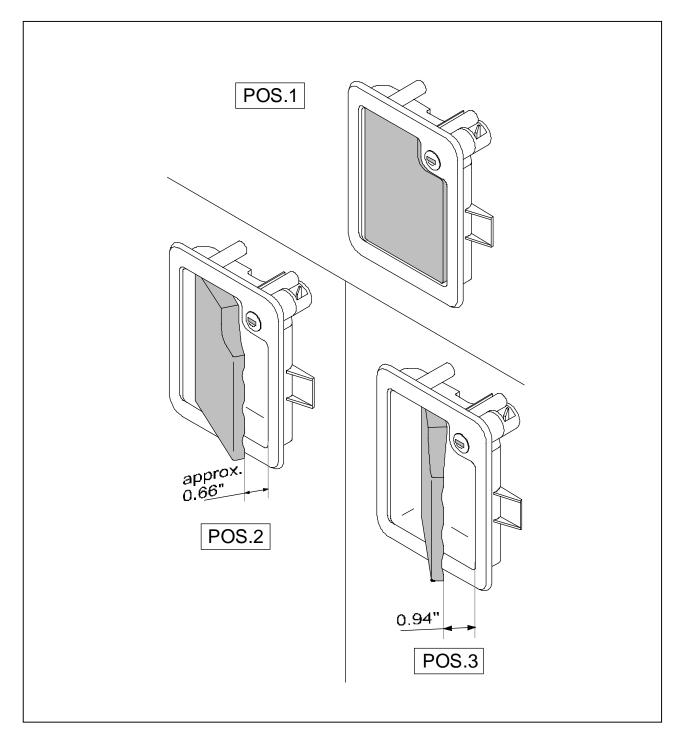
Figure 19: The three critical positions of the door lock paddle operation
