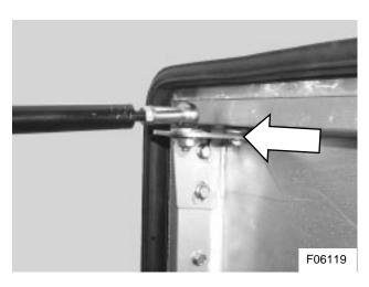
Figure 35: Additional mounting bolt and spacer.
