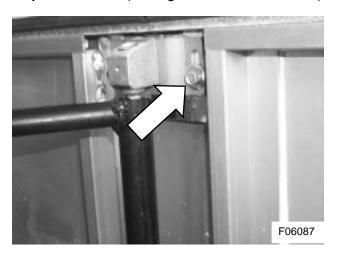
Figure 32: Height adjustable mounting brackets
