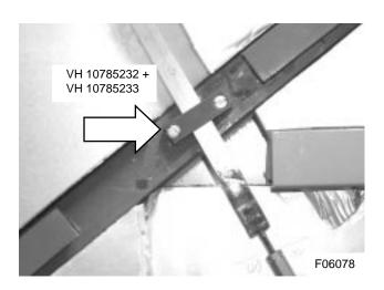
Figure 17: Emergency handle pull rod guide
