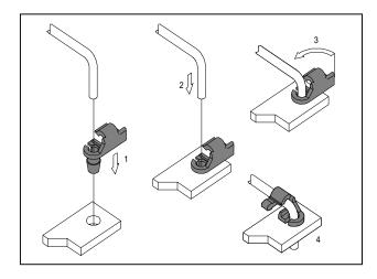
Figure 4: Snap-on rod end operation. Removal is reverse to installation
