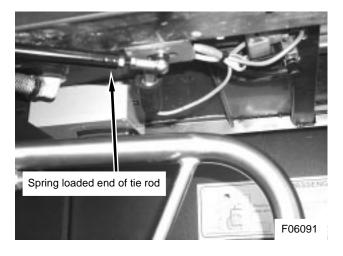
Figure 36: Tie rod installation, coach side
