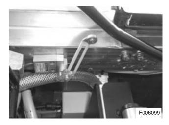
Figure 46: New location of proximity switch VH 660764615
