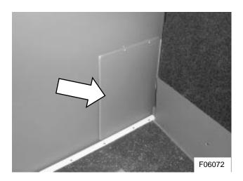
Figure 3: Door lock linkage cover panel
