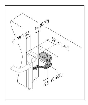
Figure 48: New switch installation dimensions (in mm and inches)
