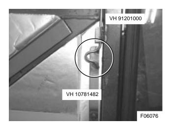
Figure 15: Push/pull rod weld
