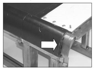
Figure 1: Mock-up showing the roof support corner bracket on which the fiberglass front cap is resting. The front cap part has been removed to show the bracket.
