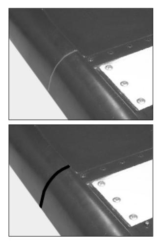
Figure 3: Gap ready to be sealed off
