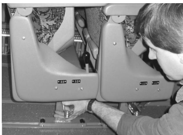
Figure 7: Securing a slider seat assembly
