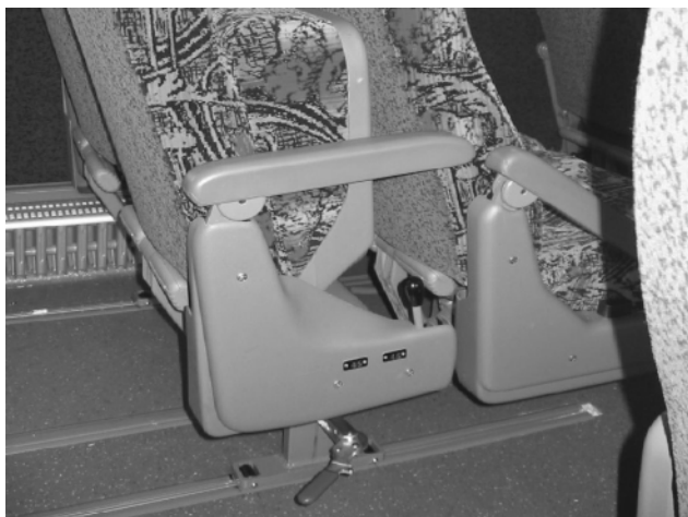
Figure 6: Seat with seat cushions pulled up and touching secure seat ahead
