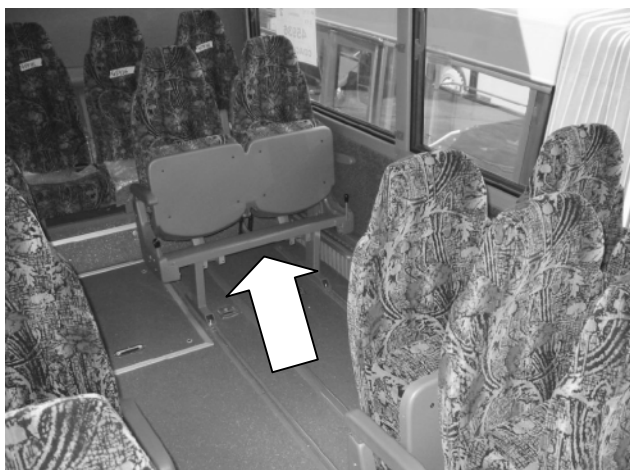
Figure 8: Seat assembly #53/54 with seat cushions folded up
