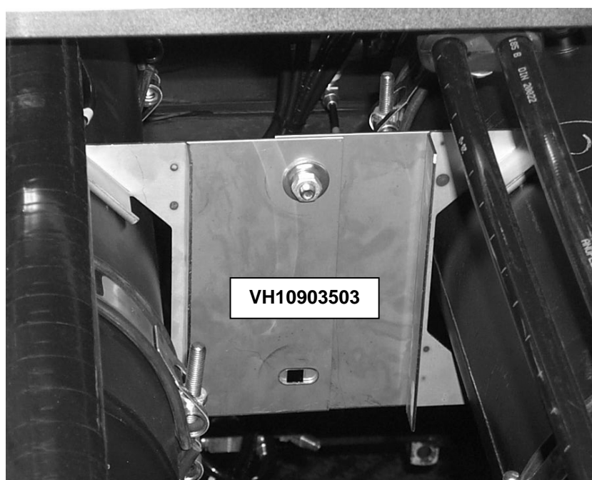
Figure 2: Tank interlocking assembly VH 10903503 for auxiliary and drive axle service brake tanks
