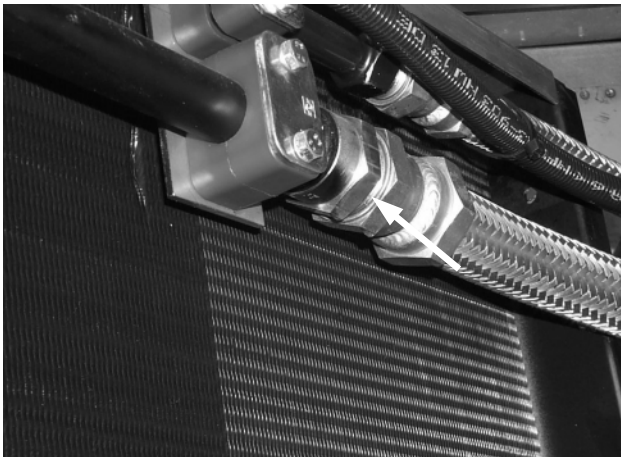
Figure 12: Condenser high pressure hose
