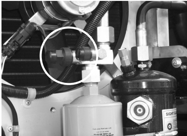
Figure 4: Filter/dryer service valve
