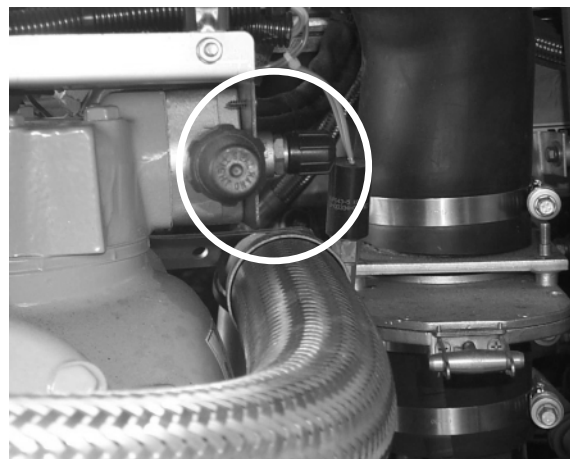
Figure 3: Discharge line (high side) service valve
