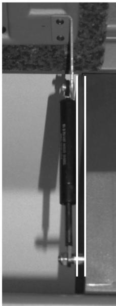
**Figure 3 (left): Gas strut parallel to parcel rack post**
