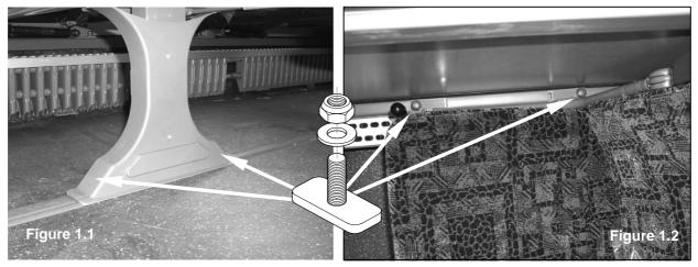
Figures 1.1 and 1.2: Passenger seat assembly - pedestal and side rail secured with tee-bolts, washers and lock nuts to coach floor and side wall tracks respectively
