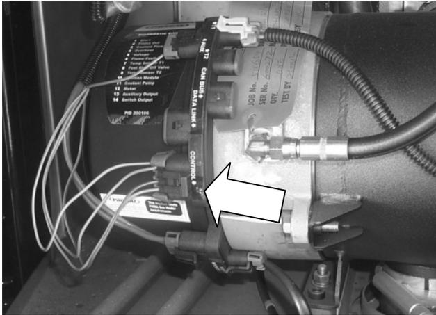
**Figure 2: Proheat M80 control connector P2 (C2045 production unit)**
