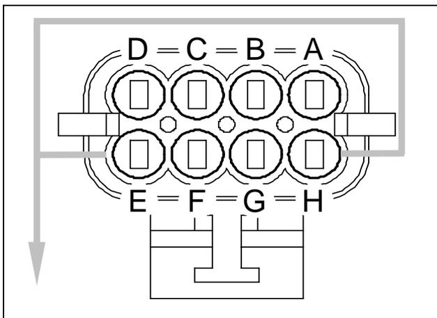
**Figure 3: P2 connector terminal location (rear view)**
