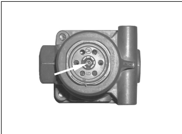
Figure 10: Pressure regulator adjusting screw
