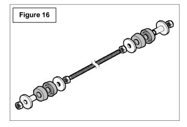
21) Complete the tie rod installation with the remaining (outer) hardware (Figures 3 and 16). Rotate and adjust the angle bracket and clamp to be parallel to the chassis anchor bracket. Adjust the tie rod length with the inner nuts.
