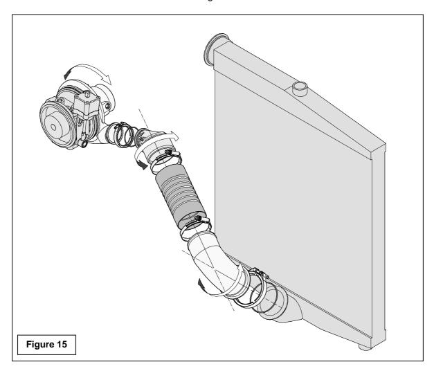
10) With the actual installation resembling the installation shown in Figure 15 as close as possible, draw reference lines on all interconnecting parts to mark their position relative to one another.
