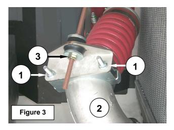
2) Undo and remove the outer nuts and mounting hardware both at the angle bracket end of the tie rod and at the chassis anchor bracket end (3, Figure 3 and Figure 4 - C2045 shown).
