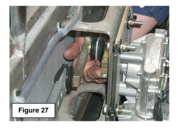
9) Reinstall the ventilation hose previously removed. Tighten the upper and lower hose clamps to a torque of 70 in.lbf (8 Nm).
