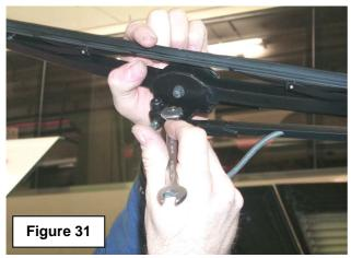
5) Turn the wiper blade in the proper direction until it is parallel to the post (Figure 32) Tighten the nut hand tight and refit the cap.
