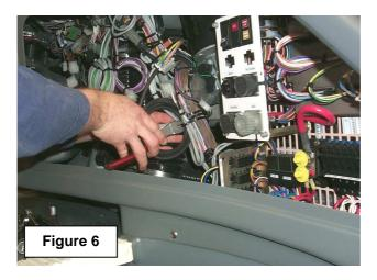
5) Detach the wiper motor multi connector (Figure 7).
