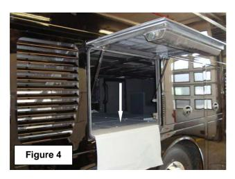
2) Working on the fire extinguisher assembly, cut loose the actuator and system (coach) cables by removing tie wraps as required.
