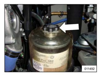
5 Locate the 12V preheater at the base of the Fuel Pro filter.
