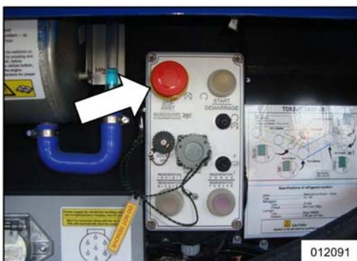
Figure 1: Safety switch on the control panel in the engine compartment (photo shows control panel of a TD925/TDX25 vehicle)
