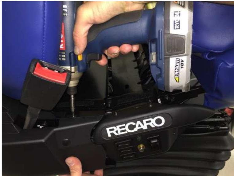
11. Replace the corner panel(s) in original position and secure with the mounting screw(s) previously removed.
