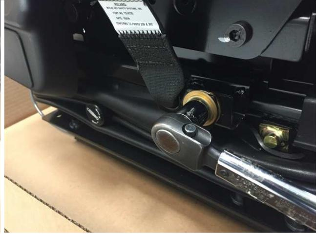
9. Route the buckle through the rear trim panel. Hand start the seat belt buckle bolt into the replacement J-Bracket part now in the seat. Torque to 50 Nm.
