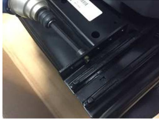
4. Position the seat back to “full forward”. Unfasten the front track bolt from the cushion frame using a 6mm hex bit and a 13mm wrench. Check the rear of seat for a track stop bolt. If present, remove it with the 6mm hex bit.
