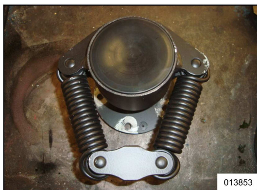
Figure 1: Crankshaft pull relief device design with two springs
