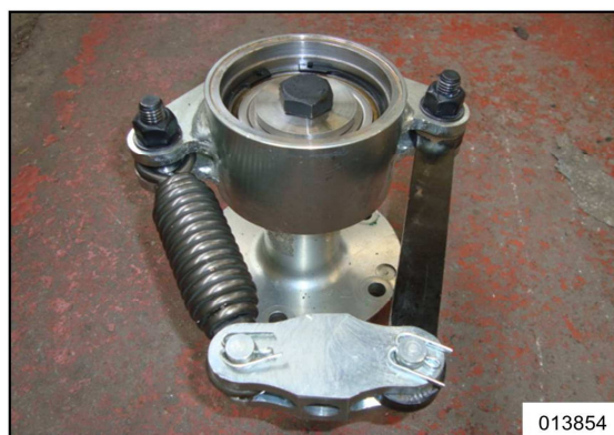
Figure 2: Crankshaft pull relief device design with one spring/tie rod
