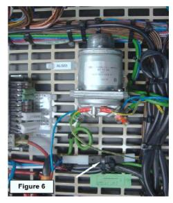
The information provided above describes how to install the fly back diode in Van Hool coaches that are equipped with Multiplex system. More information can be found in the appropriate Van Hool Service Bulletin SB1234.
