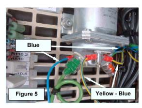
Attach the diode to the junction box grid with a cable tie as shown below
