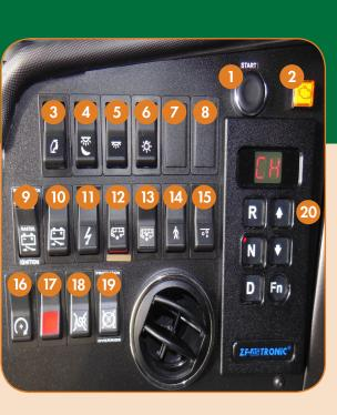
Front Kneeler Tag Axle Unloading System 16 Engine Fast Idle Emergency Engine Override Automatic Slip Reduction (ASR) 19 Retarder Foot Switch Disabler
