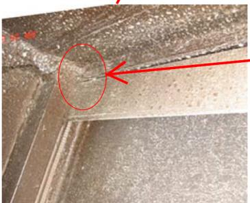
If the water is leaking into the luggage bay you will need to remove the wheel well cover and check to see if the channel in the top front corner of wheel well as shown it this picture is open with no sealer.
