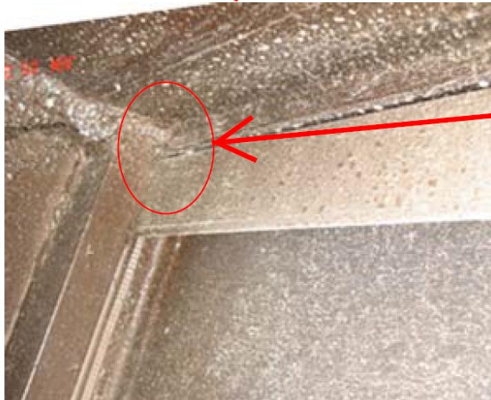
If the water is leaking into the luggage bay you will need to remove the wheel well cover and check to see if the channel in the top front corner of wheel well as shown in this picture is open with no sealer.
