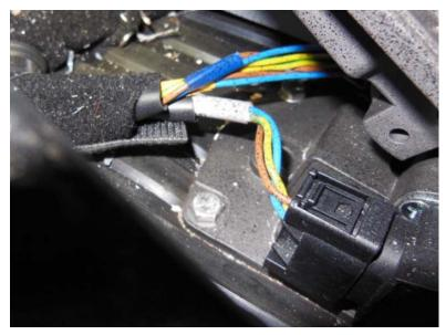
Once the pedal assembly is mounted, attach the harnesses as shown below. The connector with 3 wires attaches to the road side of the pedal assembly (kick down switch) and the connector with 6 wires (throttle position / idle validation switch) attaches to the curb side of the pedal assembly. \*\*NOTE: IF THESE CONNECTIONS ARE REVERSED, SIGNIFICANT DAMAGE WILL BE DONE TO THE PEDAL ASSEMBLY\*\*
