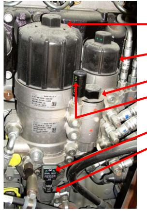
NOTE: Do not tilt the filters when removing from the housing. Possible damage to the filter or stand pipe may occur.
